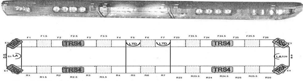
The diagram shows a long, narrow light bar with 44 LED modules. Below it is a wiring diagram with labels F1 through F26 and R1 through R20. The top row of labels (F1-F26) corresponds to the top row of LED modules, and the bottom row (R1-R20) corresponds to the bottom row. The diagram also shows four corner modules labeled TRS4 and two side modules labeled LA. The wiring diagram includes labels for the modules and their connections to a central card.
